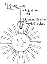
2. On a flat surface (preferably concrete) adjust both depth gauge wheel fingers until they come into contact with the surface. The box blade cutting edge should be on the same surface. This represents a "zero" inch depth. Place the measurement decal (1"- 6" yellow & black) on the side of the mounting bracket
